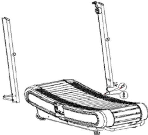
4. Attached the right hand rail to the right upright post, then fix the upper holes with 2 pcs M8\*45 screws, then fix the bottom hole with 1 pcs M8\*15 screw, then fasten all the screws. Same assembling step on the left side.
